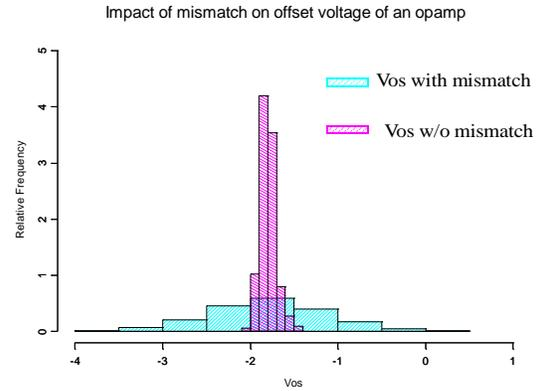
Figure 2: Distribution of  $V_{os}$  with and without mismatch
