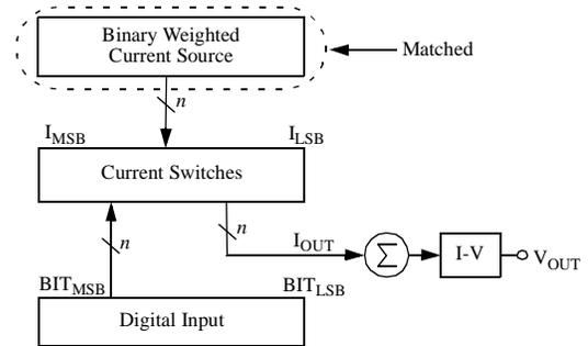
Figure 3: D/A Converter schematic
