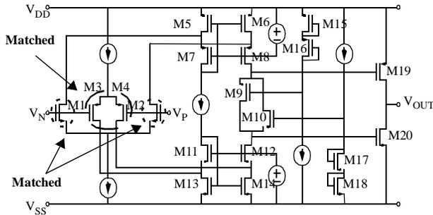
Figure 1: Low Voltage OPAMP Schematic
