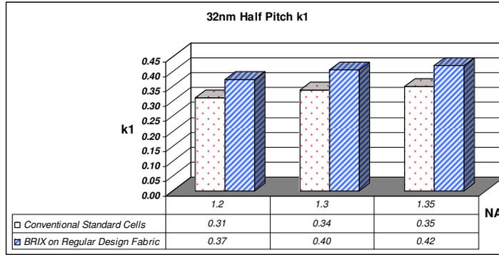
Figure 5: 32nm half – pitch  $k_1$  analysis
