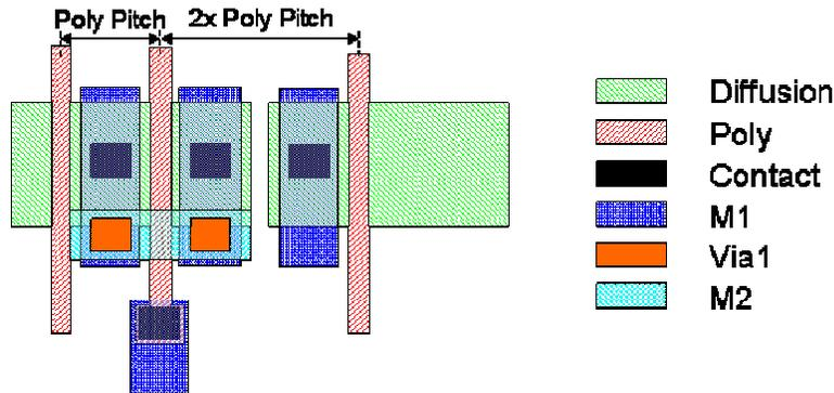
Figure 4: FEOL limited regular design fabric
