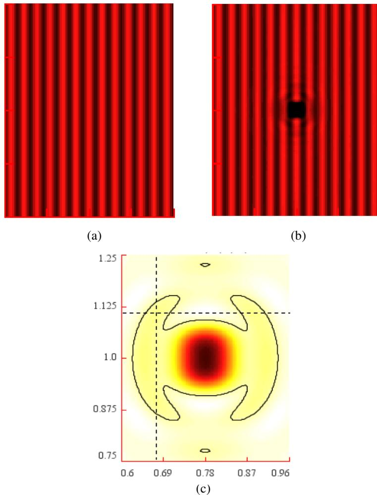
**Figure 2:** (a) Aerial image of grating (b) Aerial image of line-end in a grating (c) Zoomed in view of perturbation in aerial image caused by introducing a line-end in grating
