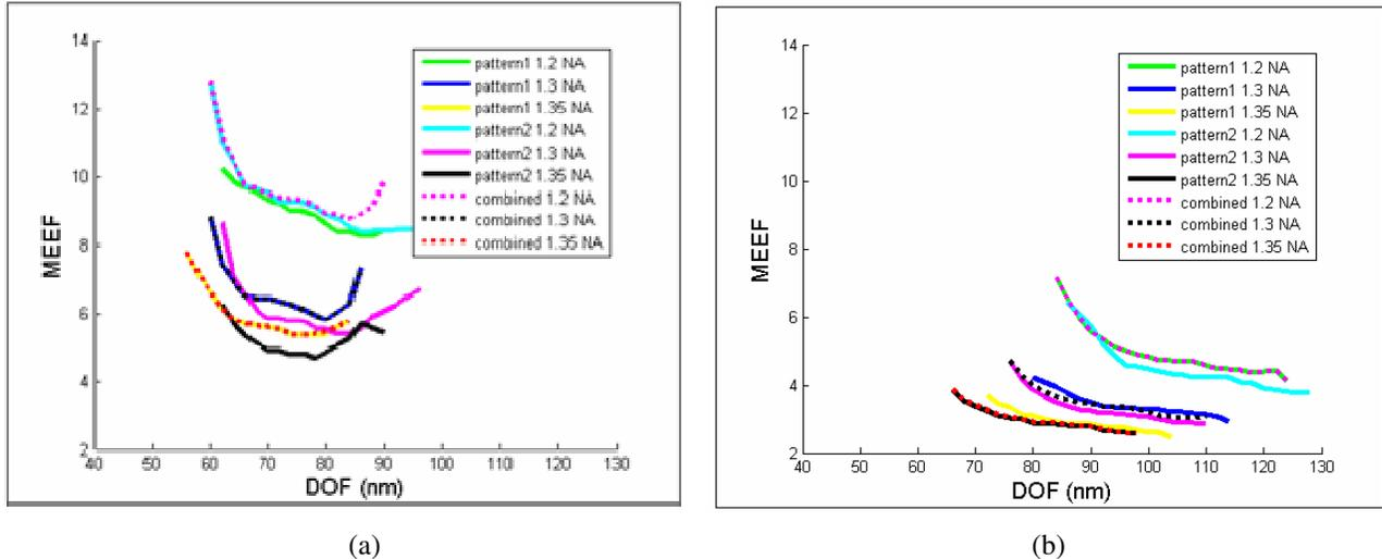
Figure 9: (a) Summary of hole simulations for standard cell (c) Summary of hole simulations for regular design fabrics
