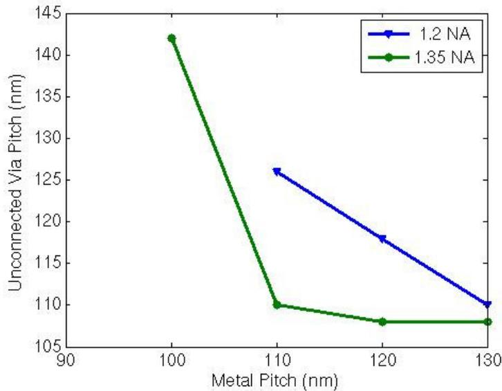
Figure 7: Summary of metal 1 line – end printability for 32nm technology node
