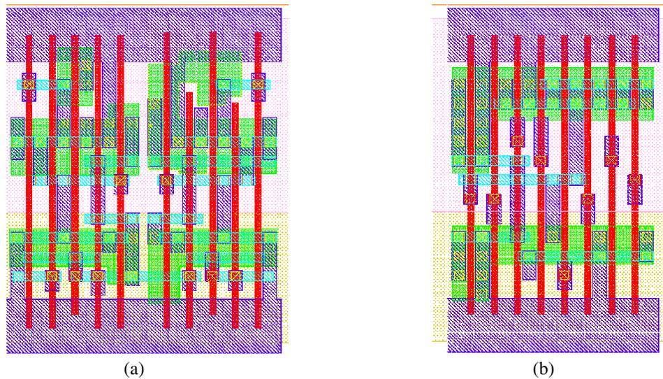
**Figure 3:** (a) Layout of brick implemented using only layout and lithography co – optimization (b) Layout of brick implemented using circuit, layout and lithography co - optimization
