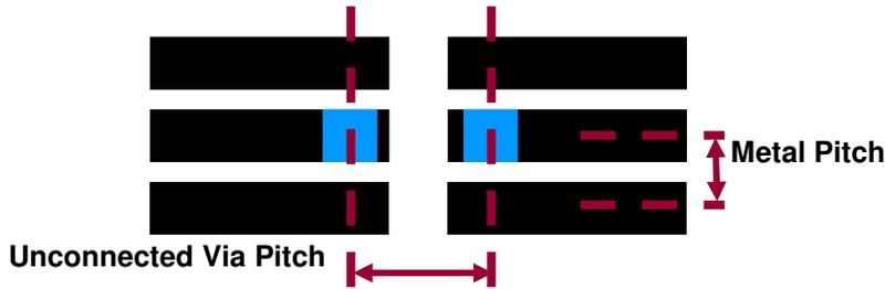
Figure 6: Unconnected via pitch for head-on line-end configuration used for the experiment
