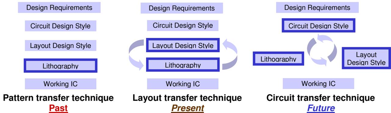
**Figure 1:** Role of lithography for past, present and future generations of IC design and manufacturing flows
