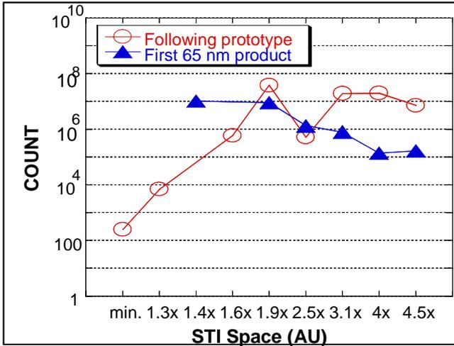
Figure 6. Comparison of the STI space use between the first 65 nm product (blue triangles) and a following prototype (red circles) in random logic. The first product did not fully exercise the random logic minimum space design rule.
