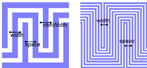
Figure 1. Schematic of Snake/Comb and "Nest" structures
