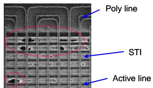
Figure 4. Top view of Poly short structures. Voids in STI can be found in the pink circles.
