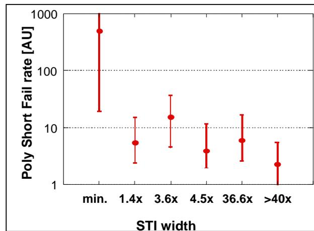
Figure 3. Poly short fail rate as a function of STI width.
