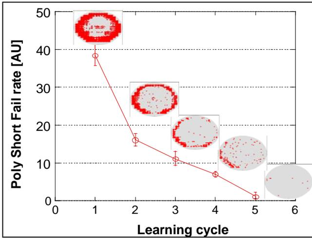
Figure 5. Reduction in Poly shorts over five process learning cycles. Red in the wafer yield maps represent failed dies.
