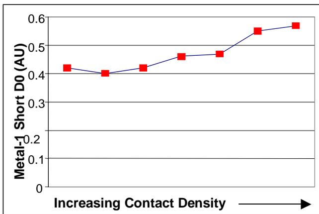
Figure 10. Metal One shorts increase as underlying Contact density increases.
