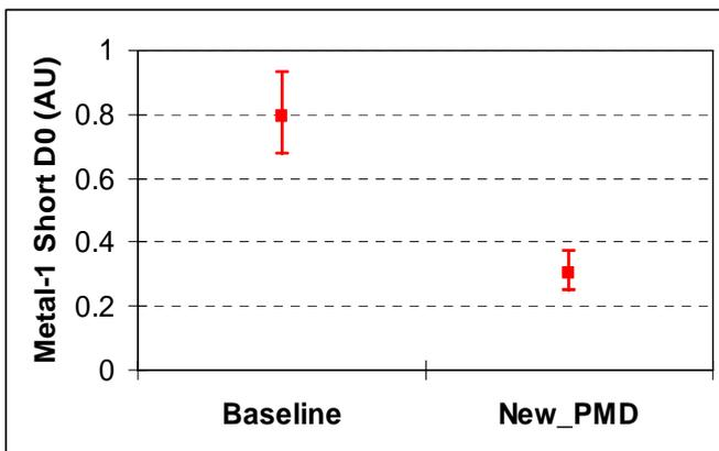
Figure 11. Comparison of Metal-1 short defectivity with "Old" and "New" PMD processes.
