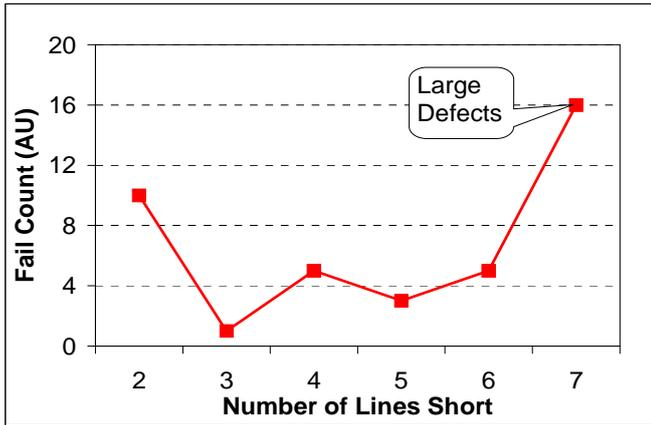
Figure 9. Metal One short defect size distribution by number of lines shorted.
