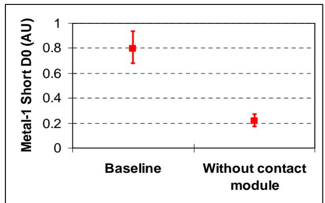
Figure 8. Comparison of Metal One short fail rate with and without Contact loop processing.
