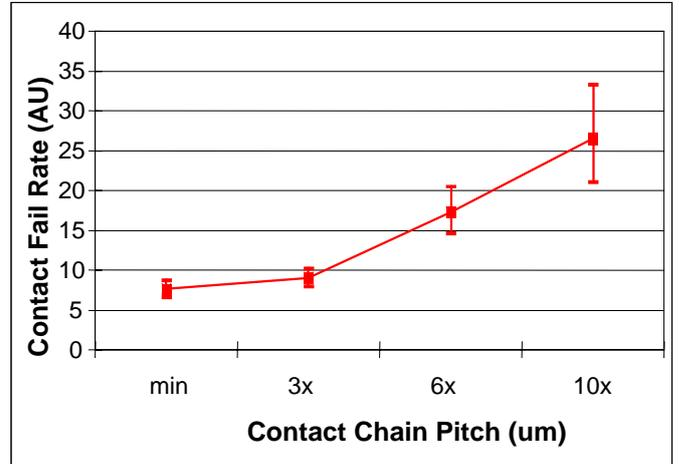
Figure 7. Increased fail rate of Contacts as a function of pitch.
