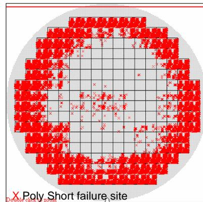
Figure 2. Fail site wafer map for Poly shorts.
