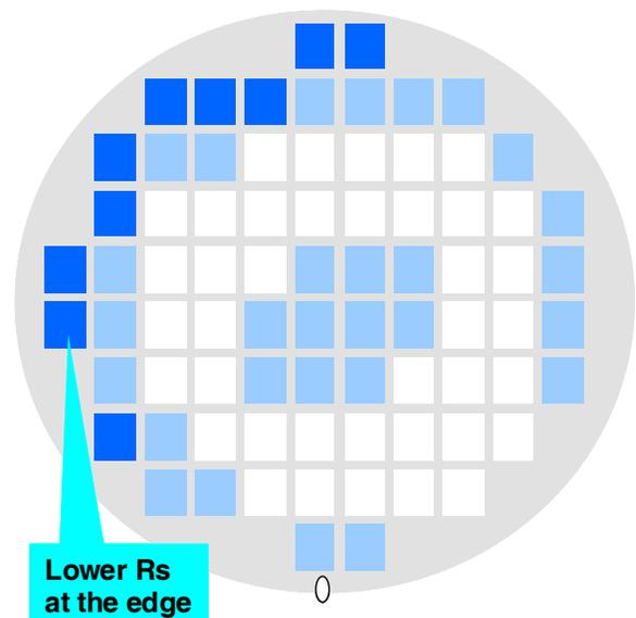
Figure 10: Detection of sheet resistance variability using Scribe CV data.
