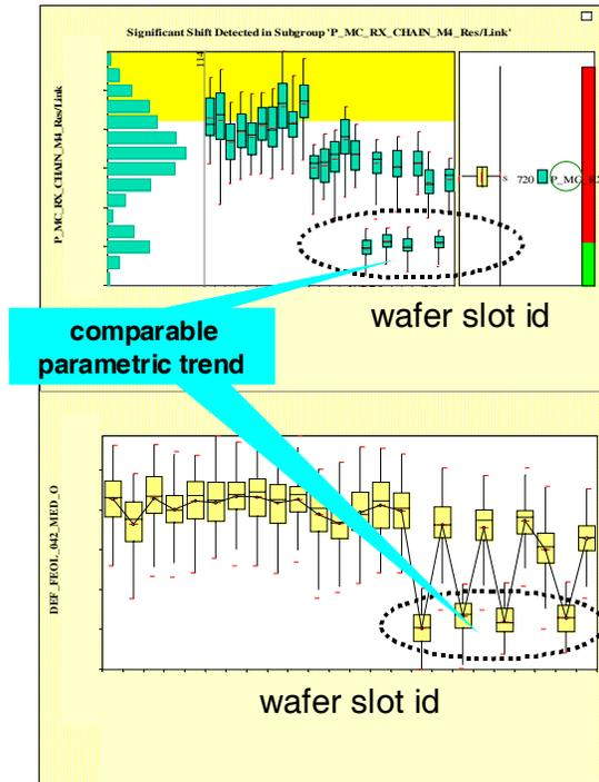
Figure 7: Comparison of detectable data trends from local interconnect chains between non-multiplexed test chips (top) and Scribe CV test chips (bottom).
