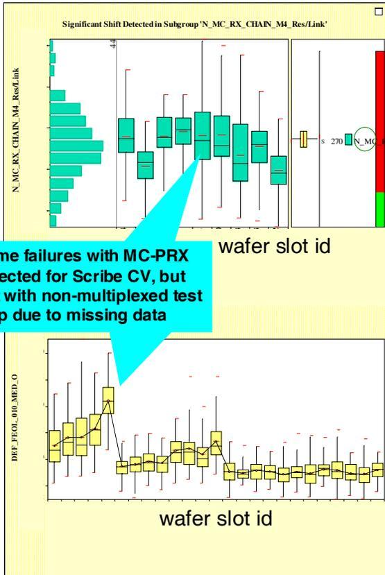
Figure 8: Data trend from local interconnect chains, which has been detected by Scribe CV test chips (bottom), but has been missed by non-multiplexed test chips (top).
