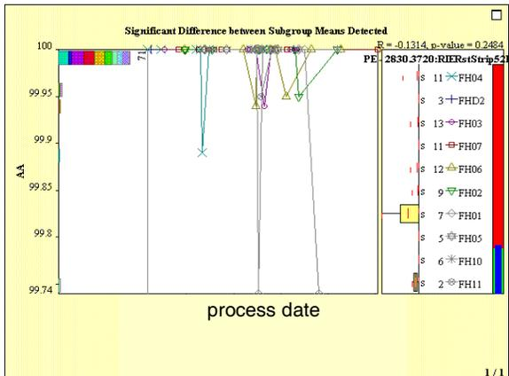
Figure 13: Spacer 2 resist dry strip tool data indicate excursions for tool FH01.
