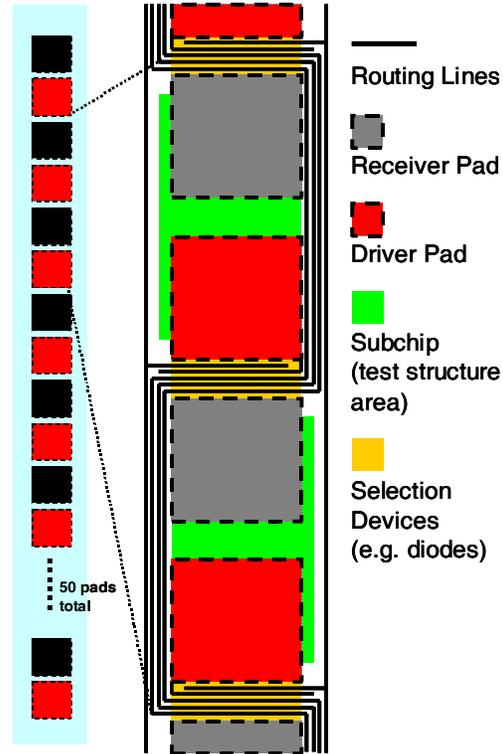
Figure 4: Arrangement of routing channels, test structures, and selection devices within the Scribe CV test chip.
