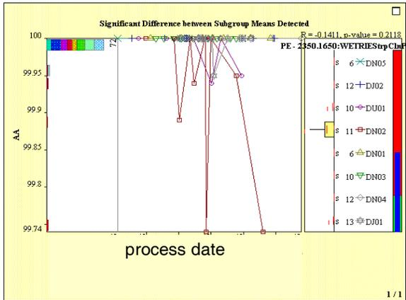
Figure 12: II dry resist strip tool data indicate issues with tool DN02.
