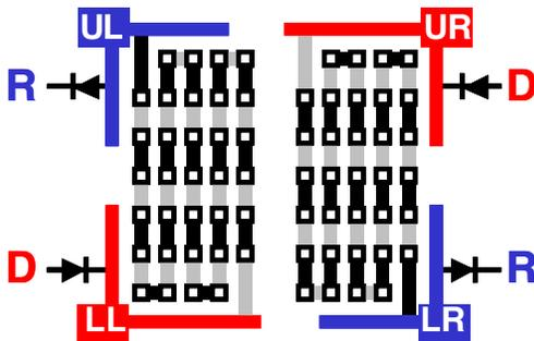
Figure 3: Placement & connection of a double contact/via chain test structure within a subchip
