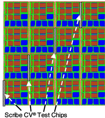
Figure 5: Example of Scribe CV test chip placement within a reticle of 16 dies.
