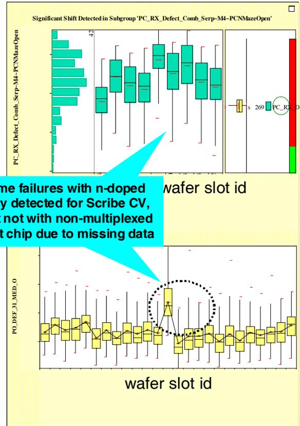
Figure 9: Data trend from n-doped poly snakes, which has been detected by Scribe CV test chips (bottom), but has been missed by non-multiplexed test chip (top).
