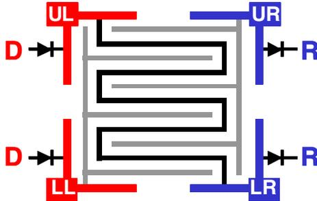
Figure 2: Placement & connection of a snake and comb test structure within a subchip
