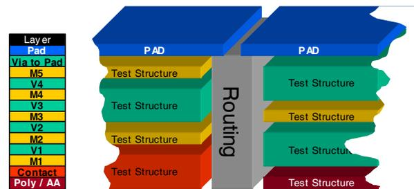
Figure 1: Concept of arranging stacked test structures under test pads.
