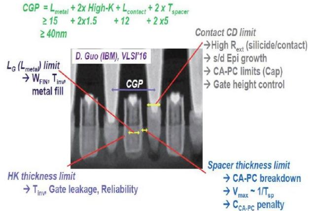
Fig. 2 Contacted Gate Pitch Scaling Challenges
