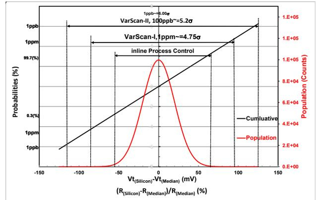
Fig. 11 VarScan I & II Parametric Defect Detection Capability
