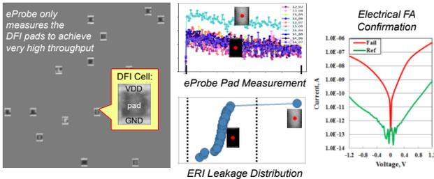
Fig. 9 eProbe Leakage Measurements Validation
