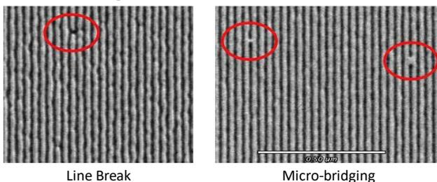
Fig 1. EUV introduces new defectivity challenges
