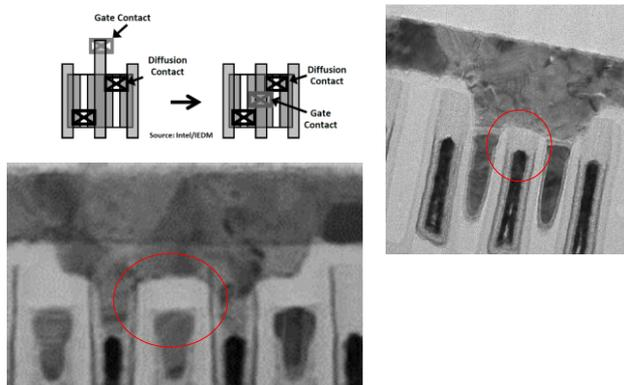
Fig. 4 Gate to S/D spacing: leakage path
