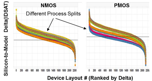
Fig. 4. Distribution of measured device performance (IDSAT) with respect to their model values for more than 2200 device layouts, NMOS and PMOS transistors. Direct Probe CV was used to collect the data from several wafers processed with different gate process conditions
