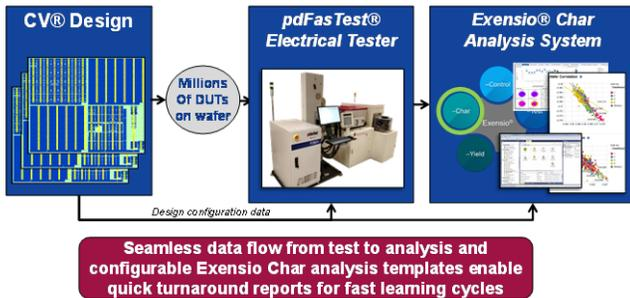
Fig. 1. Characterization Infrastructure with Characterization Vehicles, parallel tester, and Exensio analysis platform [13]
