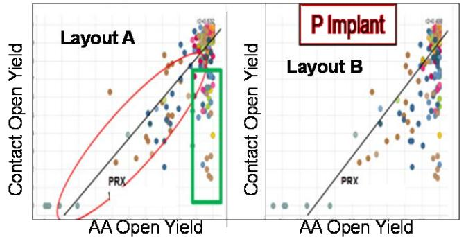
Fig. 5. Source/Drain region failure detection with a combination of Contact and Active monitor structures – correlation plots allow separation of failure modes at early development phase.
