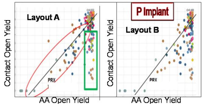
Fig. 5. Source/Drain region failure detection with a combination of Contact and Active monitor structures – correlation plots allow separation of failure modes at early development phase.
