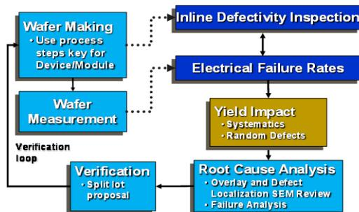
Fig. 2. Short Flow characterization loop using electrically testable structures on CV wafers.
