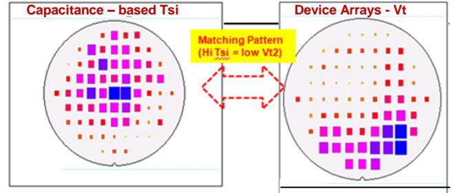
Fig. 3. Wafer level uniformity of Silicon Thickness extracted from Capacitance measurements and Vt variability in Transistor Arrays
