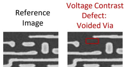
Fig. 2 Voltage contrast detected via void
