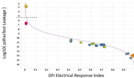
**Fig. 7** Model relating electrically measured leakage current (y-axis) and voltage contrast measured DFI ERI (x-axis) from the same test structure in scribe.
