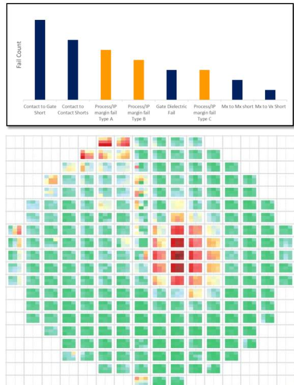
**Fig. 6** Results of DFI Fill cell measurement.
