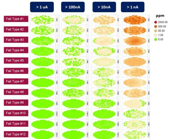
**Fig. 8** DFI Fill cell fail rates measured with various leakage thresholds.
