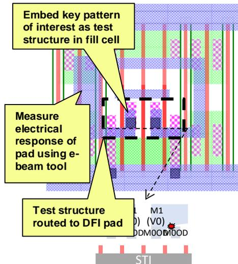
**Fig. 5** An example of a DFI Fill cell.
