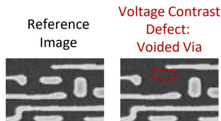
Fig. 2 Voltage contrast detected via void
